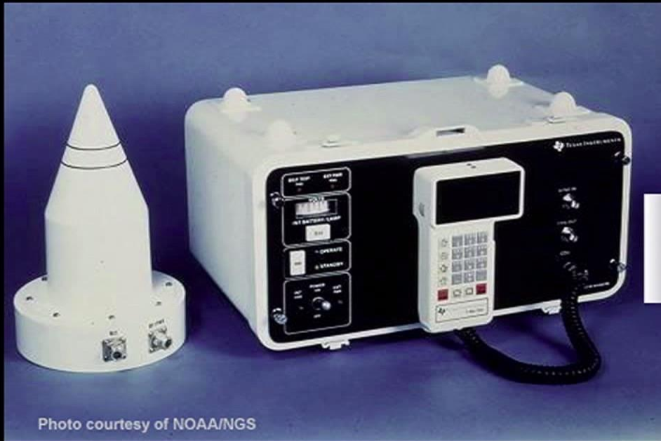
1 st commercial GPS Receiver in 1981 Weight: 53 lbs; Cost: $119,900
